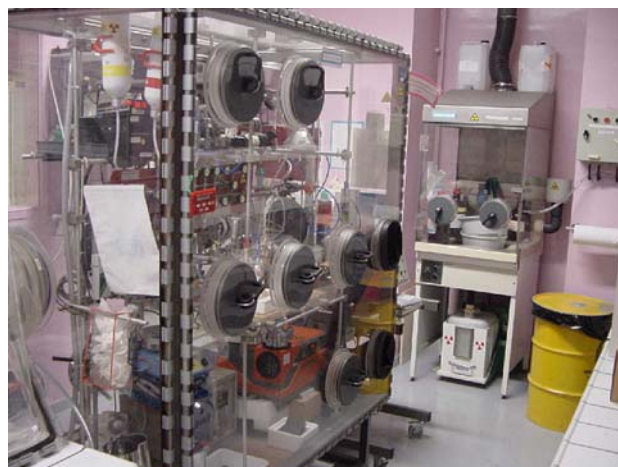
Fig. 2 Equipment for tritiation of artificial polymers at high Specific Radioactivity at the University Montpellier 1 (France)
